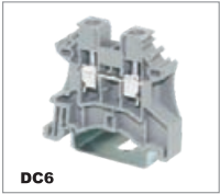
DC6 1000V/41A 0.2-10mm 2 600V/50A 22-8AWG T/W/End plate 8.0/45.0/1.5mm
