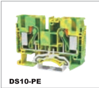
DS10-PE — 0.5-16mm 2 — 20-6AWG T/W/End plate 10.2/67.7/1.5mm
