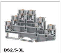
DS2.5-3L 500V/20A 0.2-4mm 2 UL 300V/20A 26-12AWG T/W/End plate 5.2/102/2.2mm
