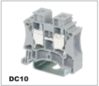
DC10 1000V/57A 0.5-16mm 2 600V/65A 20-6AWG T/W/End plate 10/43.9/1.5mm
