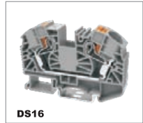
DS16 1000V/76A 0.5-25mm 2 UL 600V/85A 20-4AWG T/W/End plate 12.2/75.4/2.2mm
