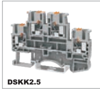
DSKK2.5 500V/22A 0.2-4mm 2 300V/20A 26-12AWG T/W/End plate 5.2/68.2/2.2mm
