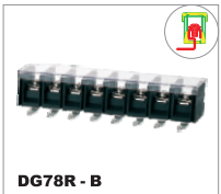
DG78R-B 750V/41A 6.0mm 2 600V40A 18-10AWG Poles 2P-20P
