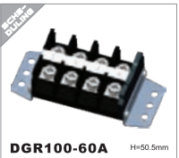
DGR100-60A H=50.5mm IEC 800V/100A 35mm 2 UL 600V/101A 20-2AWG Poles 1P-XXP
