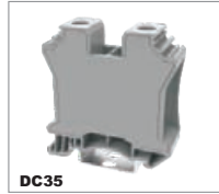
DC35 1000V/125A 2.5-50mm 2 600V/150A 14-1/0AWG T/W/End plate 16/55.4/-mm
