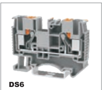
DS6 1000V/41A 0.5-10mm 2 600V/50A 20-8AWG T/W/End plate 8.2/57.7/1.5mm
