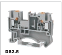
DS2.5 800V/24A 0.2-4mm 2 600V/20A 26-12AWG T/W/End plate 5.2/48.5/1.5mm
