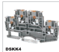
DSKK4 500V/32A 0.2-6mm 2 300V/28A 24-10AWG T/W/End plate 6.2/83.5/2.2mm
